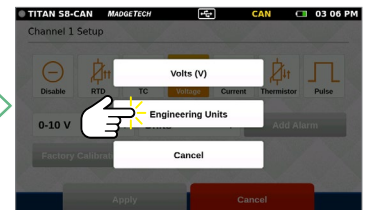
Select Engineering Units
