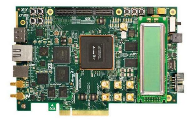
The Altera<sup>®</sup> Arria<sup>®</sup> V GX Starter Kit provides a complete design environment that includes all the hardware and software you need to develop cost-sensitive FPGA applications immediately. The development kit is RoHS compliant. The development kit features the following:
