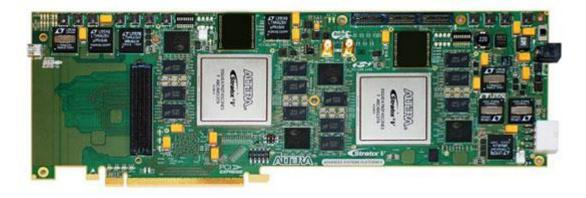
The Stratix<sup>®</sup> V Advanced Systems Development Kit is a complete systems design environment that includes both the hardware and software needed to begin architecture development and system design using Stratix V FPGAs. The PCI Express<sup>®</sup> (PCIe<sup>®</sup>)-based form-factor board combined with a one-year license for the Quartus<sup>®</sup> II software provide all that is needed to begin architecture development for a variety of applications. You can use this development kit to:
