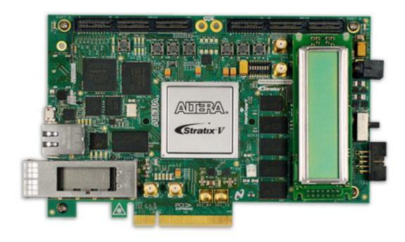
The Altera® Stratix® V GX FPGA Development Kit provides a complete design environment that includes all the hardware and software you need to begin developing FPGA designs immediately. The development kit is RoHS compliant. You can use this development kit to do the following:
