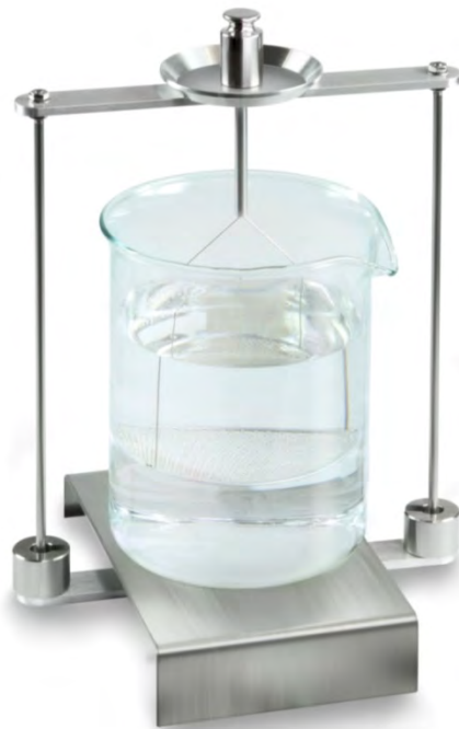
Fig.1: Density determination set YDB-03 “weighing in air” The weight of the „sample in air“ is displayed.
