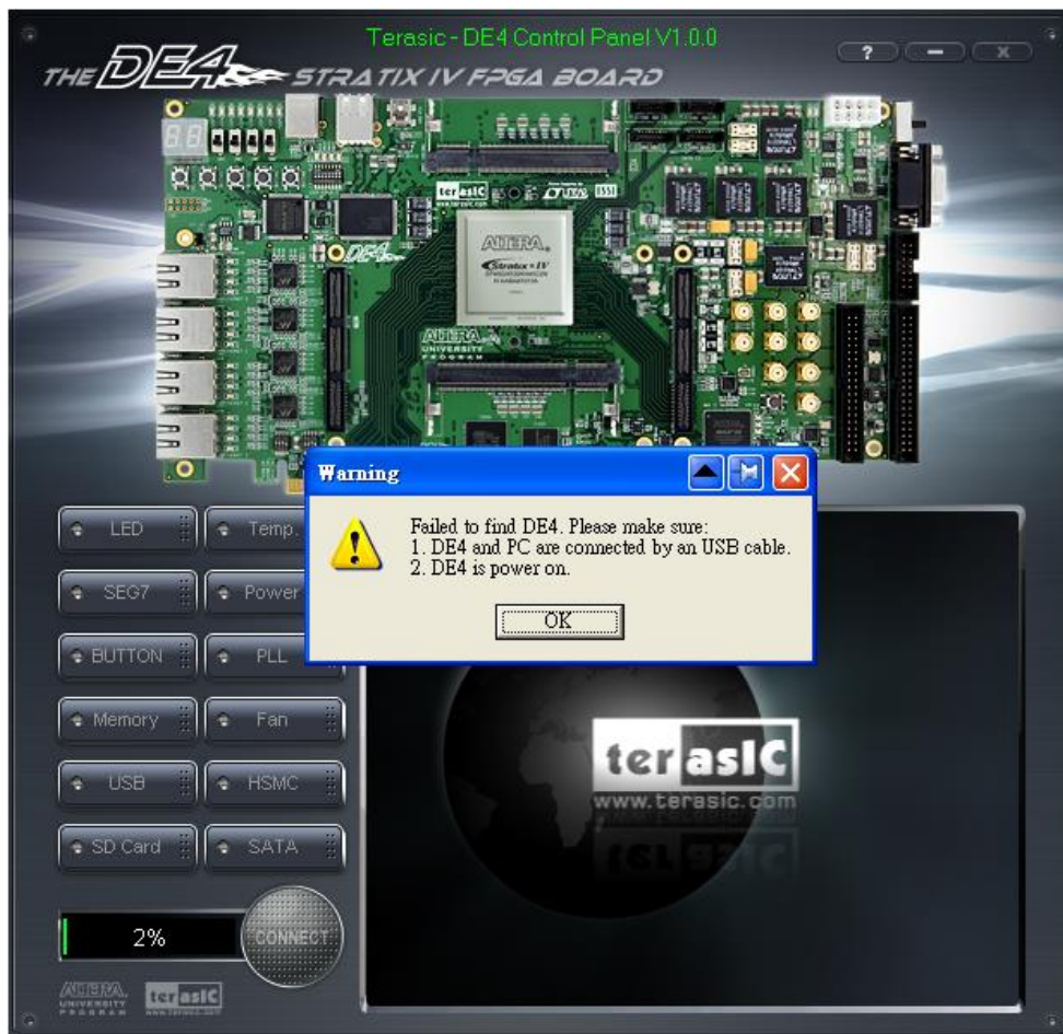
Figure 3–3 The DE4 Control Panel fails to download .sof file
