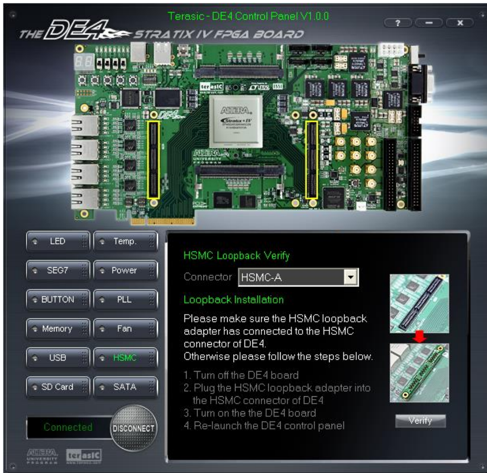
Figure 3–16 HSMC loopback verification test performed under Control Panel
