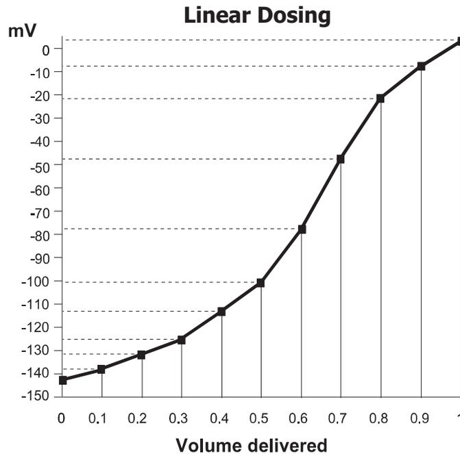
The *Linear Dosing* option is recommended for titrations with a slower reaction rate, difficult nonaqueous titrations, and specific applications.
