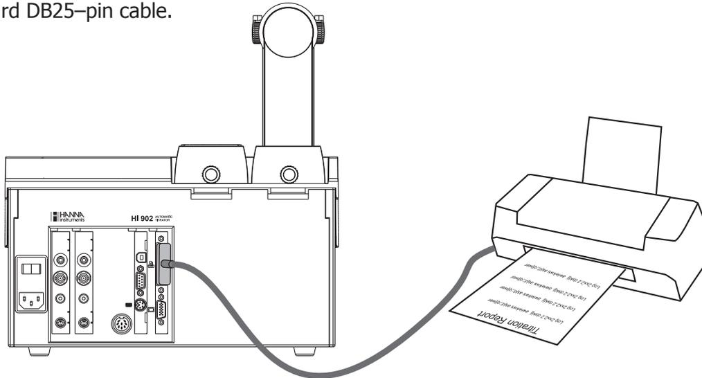
**Warning:** The titrator and the external printer must be both turned OFF before they are connected.
