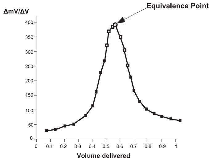
The detection algorithm looks for the maximum value of the first derivative. The first derivative must be greater than the threshold value at the maximum point (see *Recognition Options* on page 5-17).
