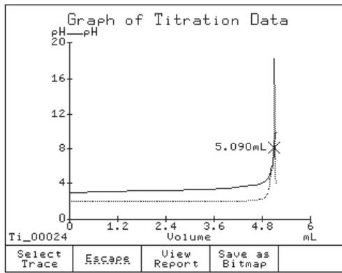
When the titration has ended, the titrator will display the equivalence endpoint volume and the final concentration of the analyte together with the **Titration Completed** message.
