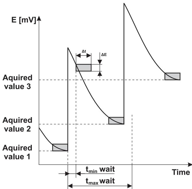
The signal stability window (condition) represents the time interval ( $\Delta t$ ) during which the potential measured in solution (mV) is confined inside the potential interval ( $\Delta E$ ). The new signal value is acquired if the stability condition is reached after the minimum ( $t_{\min}$ ) wait time.
