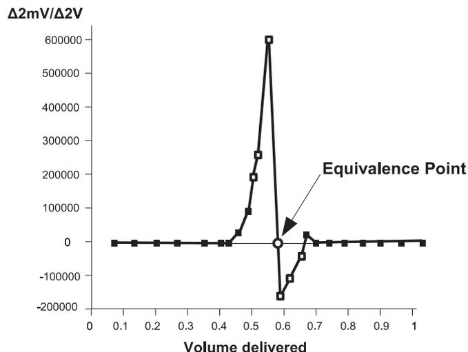
The detection algorithm looks for the point where the second derivative changes sign. The checked point, or first derivative, must be greater than the threshold value (see *Recognition Options* on page 5-17).
