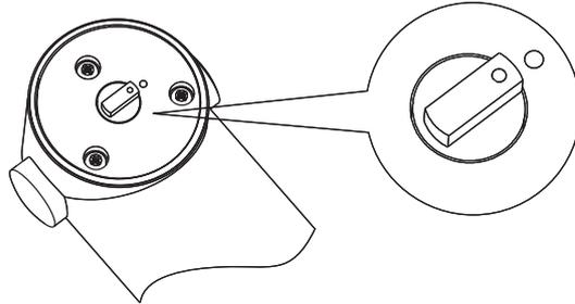
While ensuring the correct coupling between the syringe plunger (1) and the pump piston (2) (Figure 3), slide the burette into the support on the burette pump (Figure 4).
