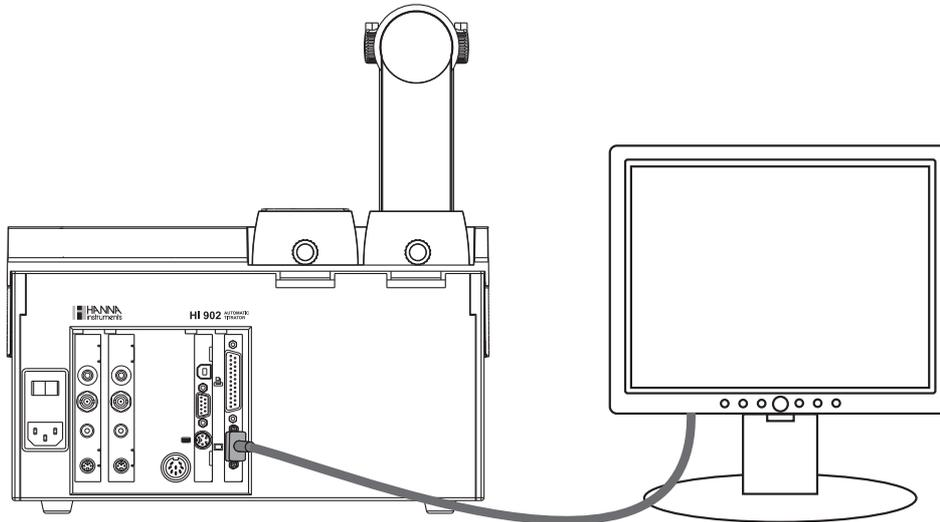
Connect the external display to the display socket.
