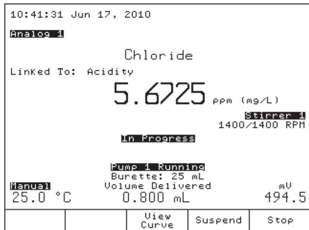
After the completion of the first titration, the selected pump will return to the home position before the second titration is started. The titrator will either start the second titration automatically or wait for user input.
