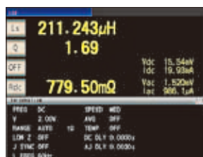
L, Q and Rdc continuous measurement screen
