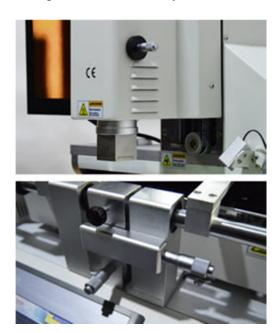
High-Precision X, Y, and  $\theta$ -Axes Alignment Micrometers
