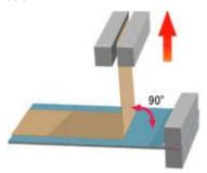
The decisive factor is the force, which is necessary to peel off the adherent, above located material.
