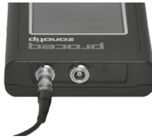
Figure 4: Connection of the 2.5 MHz transducer
