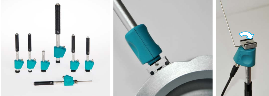
Figure 12: Overview of Equotip 550 Leeb Impact Devices and usage of support rings
