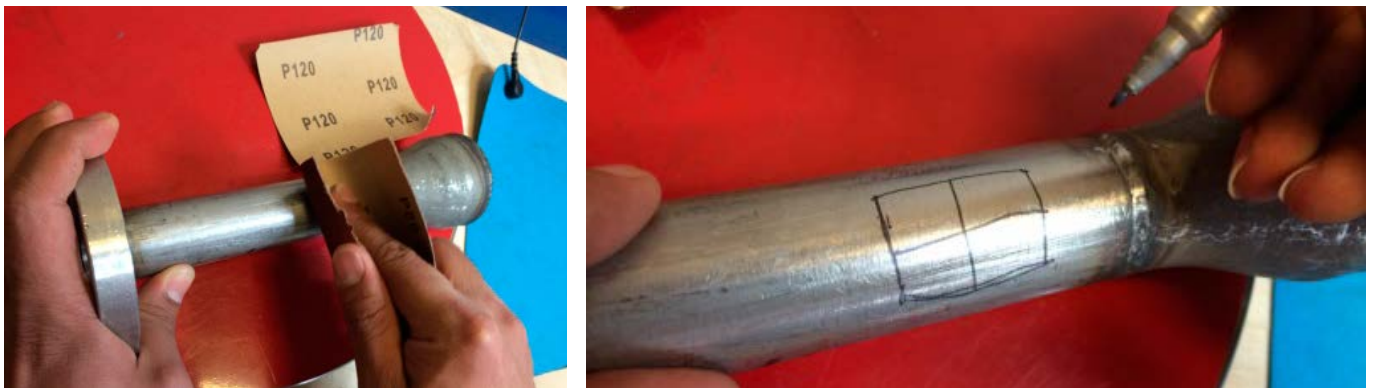
Figure 25: Preparation of test sample and marking of the test area
