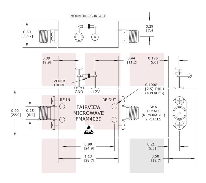
NOTE: HEAT SINK REQUIRED FOR PROPER OPERATION, UNIT IS COOLED BY CONDUCTING TO HEAT SINK.
