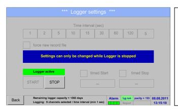
The data logger can be started without activated time settings, use the *Start* and *Stop* buttons for activate and disable. Left below there will be shown how many values are recorded and how long there still can be recorded.
