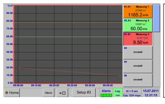
If there is no grid entered in the setup, *min* will be 0, *max* 100 and *step* 10 (Setup #3).
