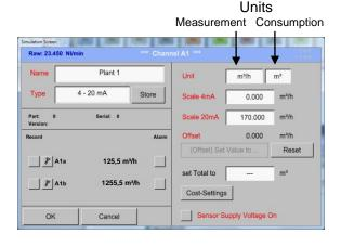
Selection of the units by pushing the text fields for the corresponding measurement and consumption units.
