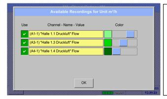
Several recordings with the same unit can be represented in one y-axis, with the help of various colour intensities.
