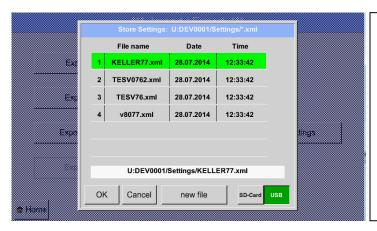
With Export system settings all existing sensor settings can be exported to a USB stick or to the internal SD card. It stores all sensor settings including recording-, alarm-, graphics-, value-and namedefintions.
