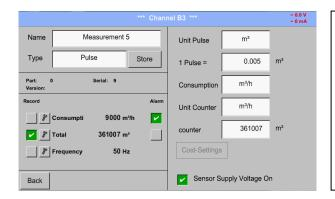
Typically the value with unit of 1 Pulse is standing on the sensor and can directly entered to the 1 Pulse = description field.
