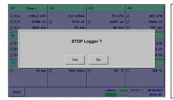
If the data logger is activated, the following window will appear and via pushing Yes it can be disabled.
