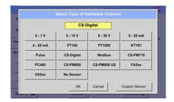
Now the *Type CS-Digital* is selected for the VA/FA 400 series and confirmed by pressing the *OK* button.
