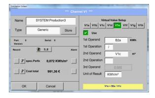
Calculation of the *specific. Perfor.* Is done in V1e with V1e = B2 / V1cFor this example it is 0,072 KWh/m<sup>3</sup>
