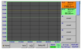
If several channels are clogged (here: 2 channels), all charts will be represented. But there is only the y-axis of the selected channel represented (here: Setup #2).
