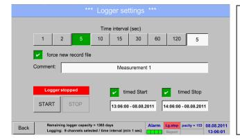
By pushing the *timed Stop* button and then the date/time description field below, the date and the stop time can be set for a data logger recording.
