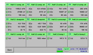
The overview of *Real time values* shows the current measured values of all connected sensors.
