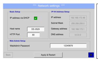
For example a *IP-Address* out of address range of the class C-Net
