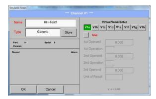
The button *Store* is implemented for storing of sensor settings (custom sensor) see <u>chapter</u> 9.3.2.11
