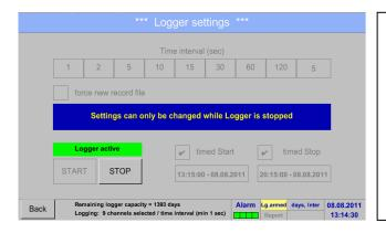
After the start and stop time activation and the created settings, the *Start* button will be pushed and the data logger is armed.
