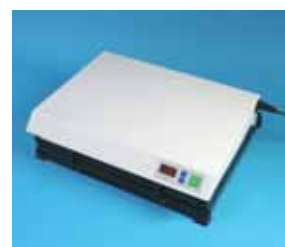
4. Exposure lid is lowered and exposure commenced.
