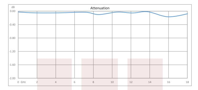
0 dB Fixed Attenuator SMA Male To SMA Female Up To 18 GHz Rated To 2 Watts With Passivated Stainless Steel Body from Fairview Microwave is in-stock and available to ship same-day. All of our RF/microwave products are available off-the-shelf from our ISO 9001:2008 certified facilities in Allen, Texas. Fairview Microwave is RF on-demand.
