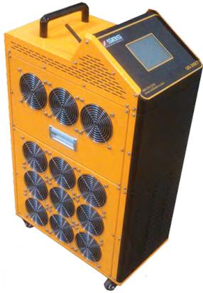
The SBS-200CT is a discharge cyler for battery testing and battery rejuvenation. The voltage range of 24–96 Vdc covers many types of traction batteries including: stationary, forklifts, automobile, golf cart, train, wheel chair, etc. When equipped with an industrial charger (sold separately), the SBS-200CT can provide an unmanned discharge/cycling solution to help increase battery capacity. The unit includes wireless modules for individual cell readings and software to generate detailed reports.
