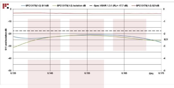
High Power Circulator SMA Female With 20 dB Isolation From 135 MHz to 175 MHz Rated to 150 Watts from Fairview Microwave is in-stock and available to ship same-day. All of our RF/microwave products are available off-the-shelf from our ISO 9001:2008 certified facilities in Allen, Texas. Fairview Microwave is RF on-demand.
