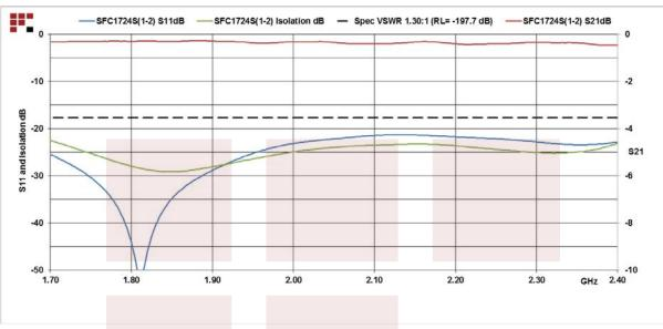
Circulator SMA Female With 17 dB Isolation From 1.7 GHz to 2.4 GHz Rated to 10 Watts from Fairview Microwave is instock and available to ship same-day. All of our RF/microwave products are available off-the-shelf from our ISO 9001:2008 certified facilities in Allen, Texas. Fairview Microwave is RF on-demand.
