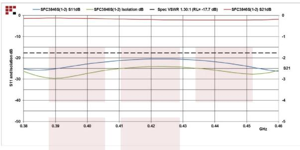
High Power Circulator SMA Female With 20 dB Isolation From 380 MHz to 460 MHz Rated to 1000 Watts from Fairview Microwave is in-stock and available to ship same-day. All of our RF/microwave products are available off-the-shelf from our ISO 9001:2008 certified facilities in Allen, Texas. Fairview Microwave is RF on-demand.
