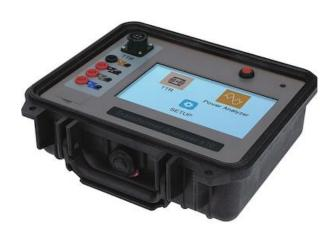
TEKON610 is a system designed for distribution (service) transformer, which not only measures electrical conditions such as turns ratio, excitation current, power, harmonics and inrush current, but also tests transformer's electrical characteristics.
