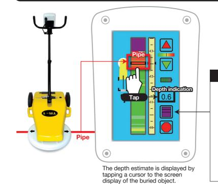
The display screen visualizes having pipe line or not under the ground with red, yellow and green.
