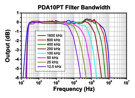
Figure 4 PDA10PT Filter Bandwidth (50 Ω Load)
