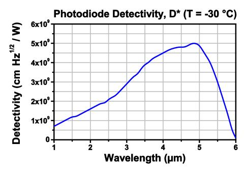
Figure 3 PDA10PT Photodiode Detectivity (D\*) at 0 dB Gain Setting
