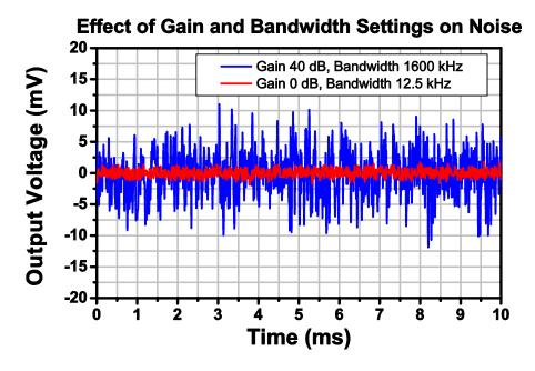
Figure 5 Noise Comparison at Min and Max Gain and Filter Settings
