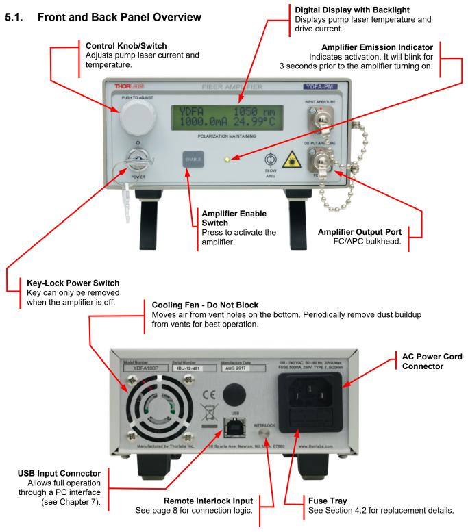
Figure 1 Front and Rear Panels of the YDFA100P Fiber Amplifier (YDFA100S Does Not Have Polarization Features)
