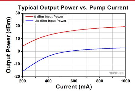
Figure 2 Output Power Versus Pump Current, for 0 dBm and -20 dBm Input Powers at 1050 nm
