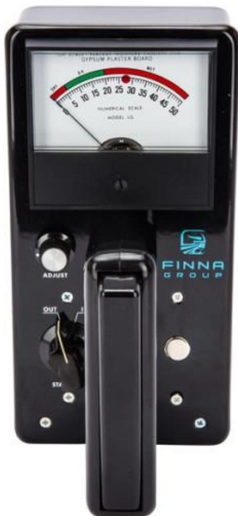
This single range instrument uses the Radio Frequency Capacitance Method to measure the moisture content of Gypsum Wallboard. Color Coded direct reading dial for fast comparison. Has a range of 0 to 25% and is operated from a single rechargeable NiMH battery. It gives the operator an average moisture content down to a penetration of one inch. The LG uses Stainless Steel Buttons that make contact with the board. Complete with a Carrying Case, NiMH Battery and Operating Instructions Book.
