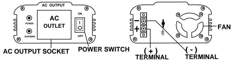
IF THE TOTAL WATTS OF ELECTRICAL APPLIANCES EXCEEDS THE OUTPUT CAPACITY OF INVERTER. OR AFTER OPERATING FOR A PERIOD OF TIME. IF THE TEMPERATURE OF THE INVERTER REACHES 60 DEG C, THE INVERTER SHALL BE REDUCED AC OUTPUT BY THE PROTECTION CIRCUIT.
