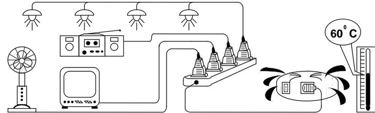
WHEN CONNECTED TO ANY APPLIANCE, BE SURE TO TURN ON INVERTER FIRST. AND THEN TURN ON THE POWER SWITCH OF THE APPLIANCE.
