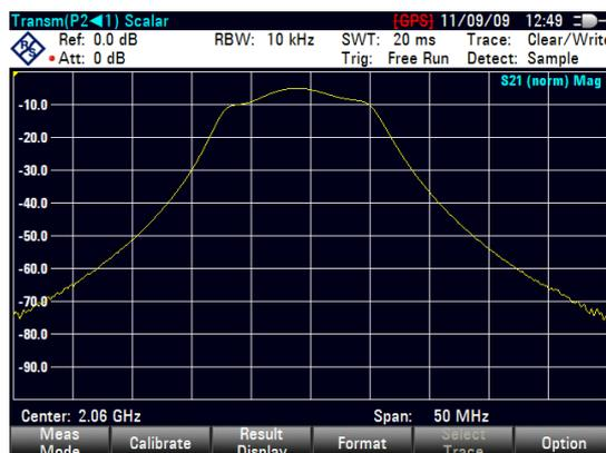
You can change the measurement configuration (e.g. select another sweep time or detector) without affecting the accuracy of the measurement except the frequency parameters and attenuation.
