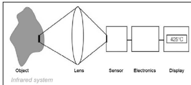
**Figure 30:** Main principle of noncontact thermometry
