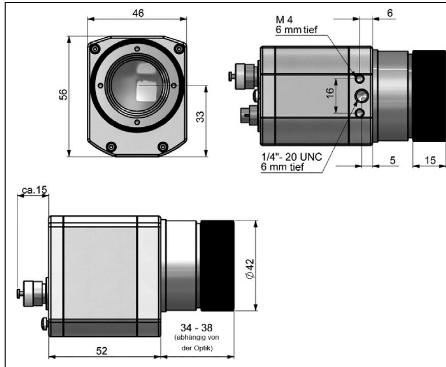
**Figure 7:** PI400/ PI450/ PI450G7/ PI640/ PI1M, dimensions [mm]
