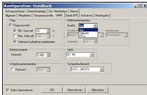
**Figure 36:** Adjustment of the emissivity in the software PI Connect (menu Configuration/ Device)
