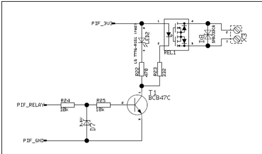
**Figure 41:** Relay output at industrial PIF
