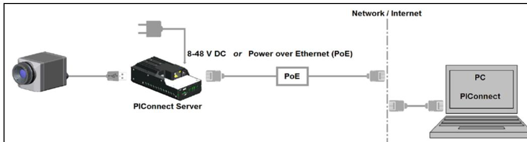
**Figure 23:** Ethernet network communication with PI Netbox
