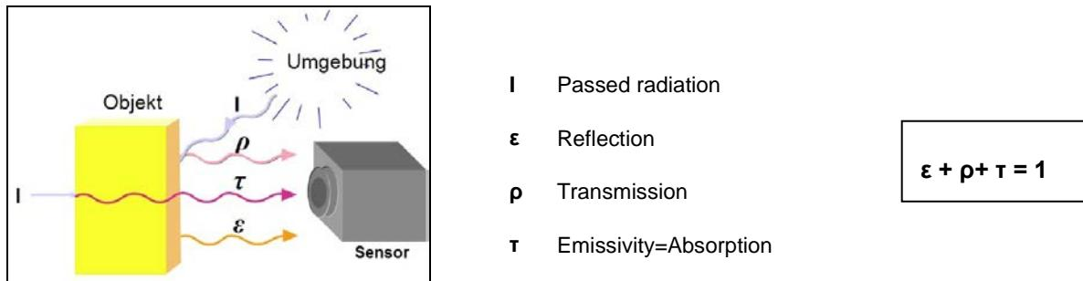
**Figure 32:** Capability of an object to emit radiation
