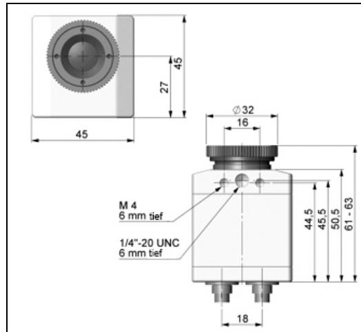
Figure 5: PI160, dimensions [mm]
