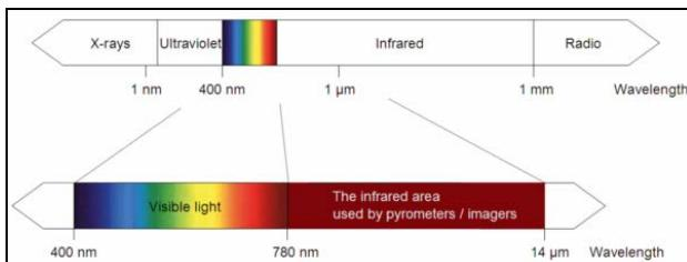
**Figure 29:** The electromagnetic spectrum and the area used for temperature measurement
