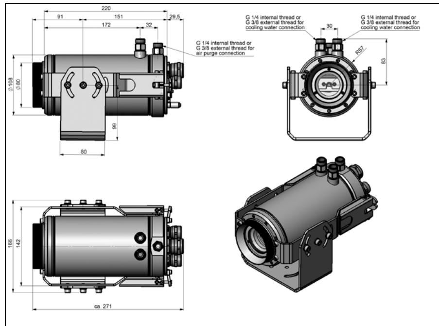
**Figure 13:** Cooling Jacket Advanced [Part No.: ACPIxxxCJAS], Standard Version, 38°/ 62° optics - Dimensions
