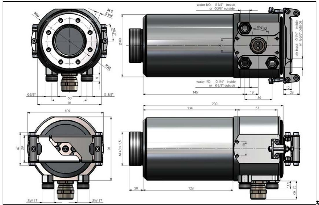
**Figure 10:** Cooling Jacket - Dimensions
