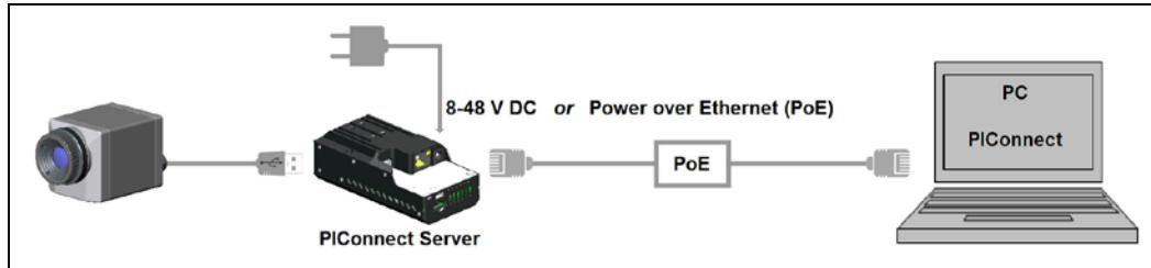
**Figure 22:** Ethernet direct communication with PI Netbox
