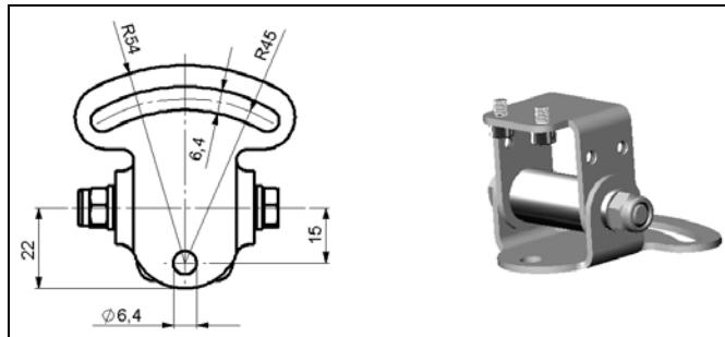
**Figure 8:** Mounting base, stainless steel, adjustable in 2 axes [Part No.: ACPIMB]
