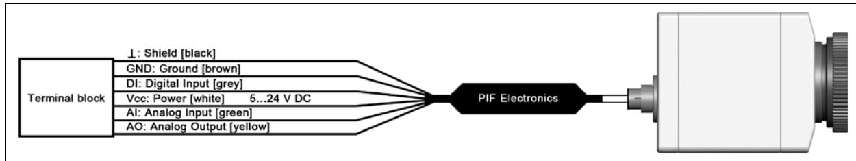
**Figure 16:** Configuration Standard Process Interface (PIF)
