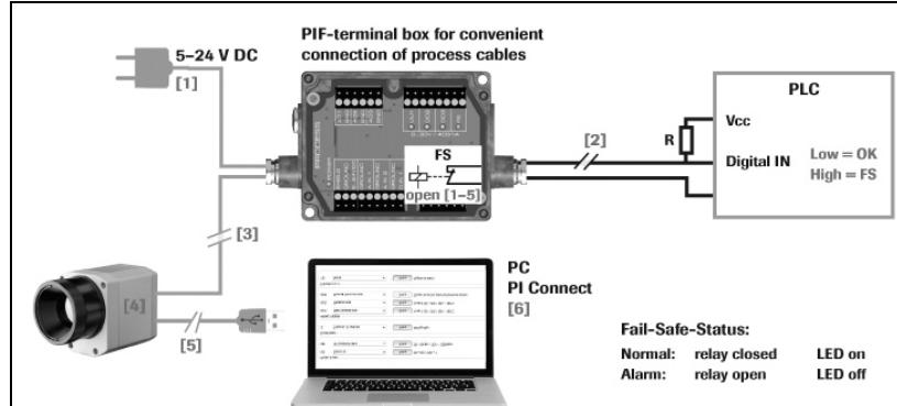
Figure 20: Fail-Safe monitoring states
