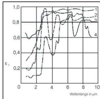
**Figure 33:** Spectral emissivity of several materials: **1** Enamel, **2** Plaster, **3** Concrete, **4** Chamotte
