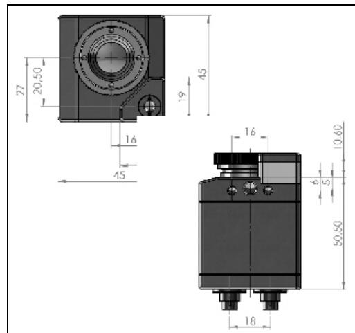
Figure 6: PI200/ 230, dimensions [mm]
