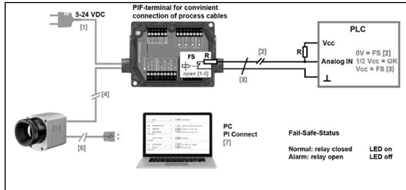
**Figure 21:** Fail-Safe monitoring states
