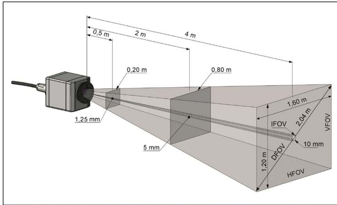
**Figure 4:** Measurement field of the infrared camera PI representing the  $23^\circ \times 17^\circ$  lens
