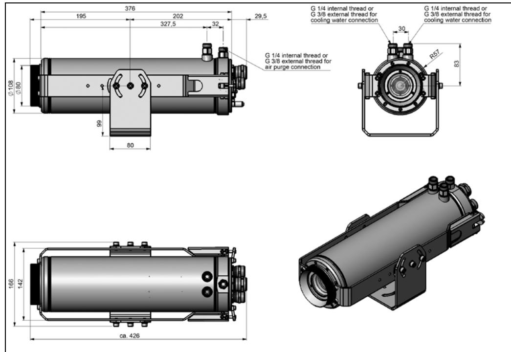
**Figure 14:** Cooling Jacket Advanced [Part No.: ACPIxxxCJAE], Extended Version, 38°/ 62° optics - Dimensions
