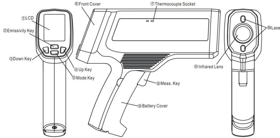
display the surface temperature. The Distance:Spot is 100:1. The two laser points are the reference for the target spot size. Please make sure the target area is within the field of view.
