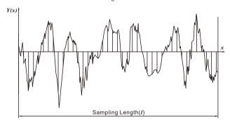
9.2.2 Rz maximum height of profile Sum of height of the largest profile peak height **Ypmax** and the largest profile valley depth **Yvmax** within a sampling length.
