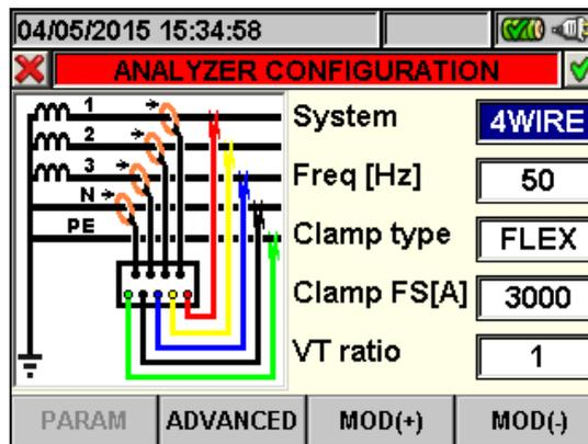
Fig. 44: Analyzer configuration screen for 4-wire system – ENG\_UK type
