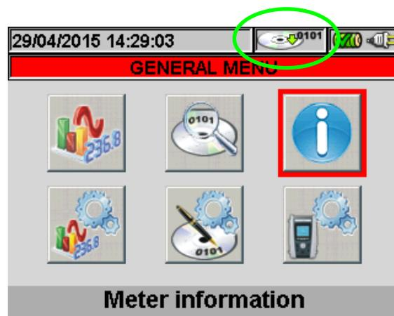
Fig. 79: Meter in recording run
