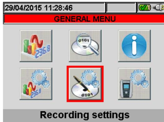
Fig. 62: Recording Settings screen selection
