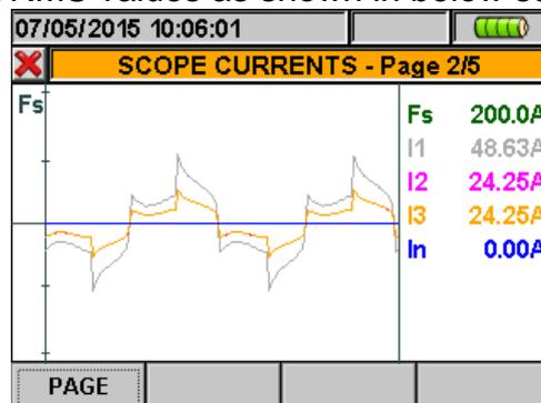
Fig. 28: Current waveforms screen for 4-wire systems
