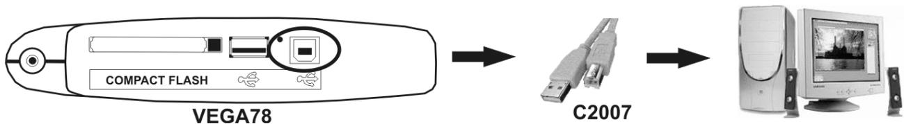
Fig. 112: Connection of meter to PC
