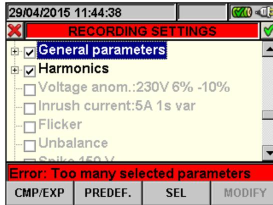
Fig. 67: General Parameters section: too many selected parameters
