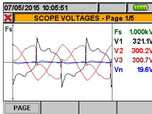
Fig. 27: Voltage waveforms screen for 4-wire systems
