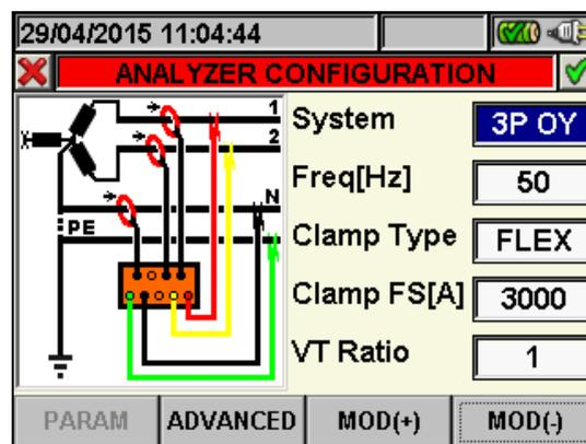
Fig. 60: Analyzer Configuration screen for 2-phase system 3-wire 3P OY – ENG\_UK type
