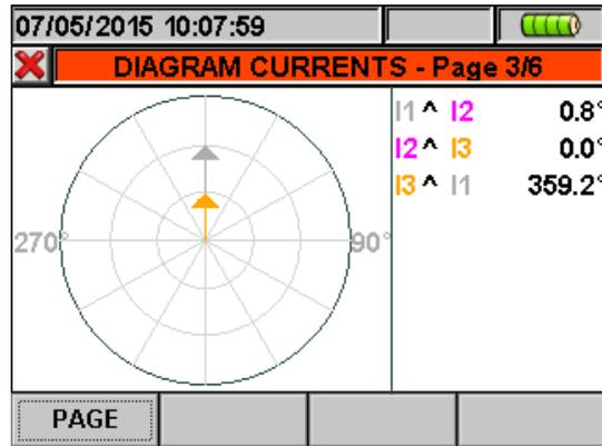
Fig. 40: Vectorial current diagram for 4-wire system
