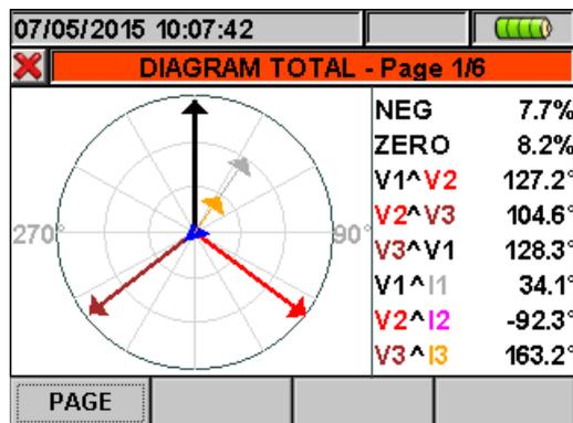
Fig. 38: Vectorial diagram total for 4-wire system
