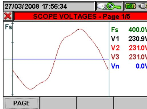
Fig. 100: Voltage scope in three-phase 4-wire system
