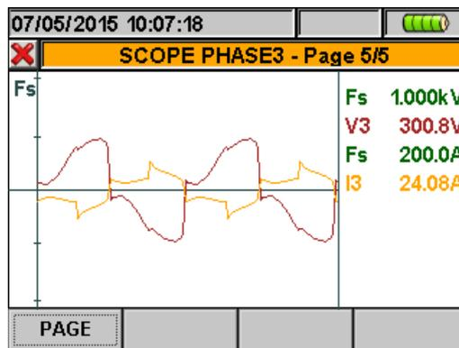
Fig. 31: Voltage/Current waveforms screen L3 phase for 4-wire systems
