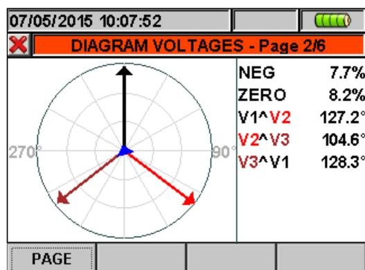
Fig. 39: Vectorial voltage diagram for 4-wire system
