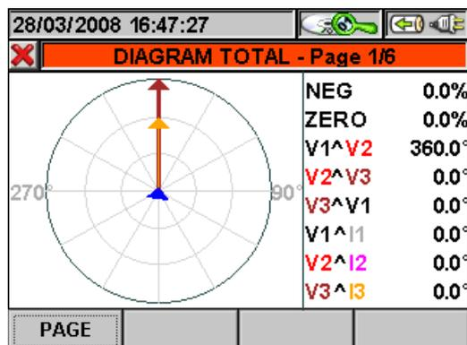
Fig. 102: Total vector diagram in three-phase 4-wire system
