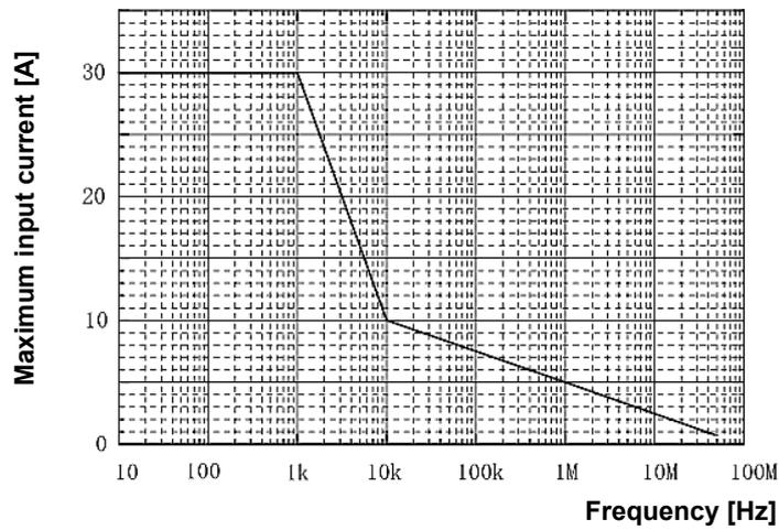
**Figure 2 Derating according to frequency**
