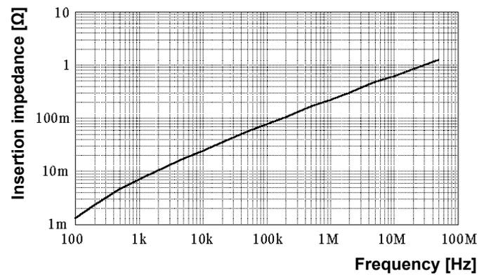
**Figure 3 Input impedance (typical)**
