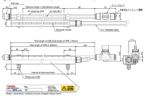
The maximum length of HPB total length for single air assist bar is 1500mm. Alternating installation of AAB for longer HPB.
