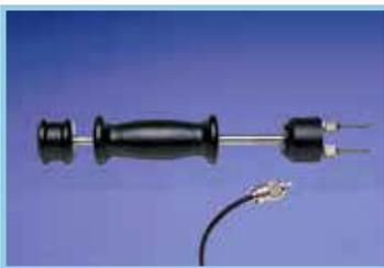
The #496 2" insulated pins on this slide hammer electrode allow you to determine accurate moisture readings at various levels of penetration. Useful for determining moisture gradients in lumber.
