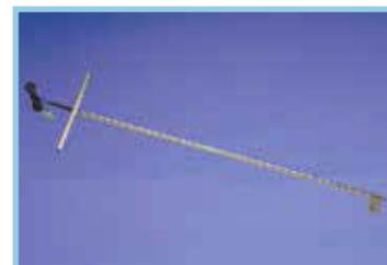
T-handle electrode with 3/8" penetration to check moisture in stacks of lumber in or out of the kiln. Stickers must be at least 5/8". Also available in 4 1/2 ft. length as 42E/B/4.5.
