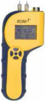
The RDM-3 is a handheld moisture meter packed with features and is perfect for the lumber and woodworking industries. The RDM-3 is ideal for anyone who needs to collect and analyze key statistical information, and features a menu driven display, corrections for 69 individual wood species, and temperature correction. Once stored, your data can be downloaded to Excel spreadsheet using optional computer software.
