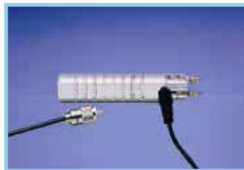
Uses the same contact pins that are mounted on each meter, providing 5/16" penetration. Used on wood up to an inch thick.
