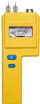
A tried and true solution for woodworkers and small shops, the J-4 is a user friendly meter that you'll pick up with ease, but never want to put down! The J-4 features an easy to read analog display, and built-in calibration check.
