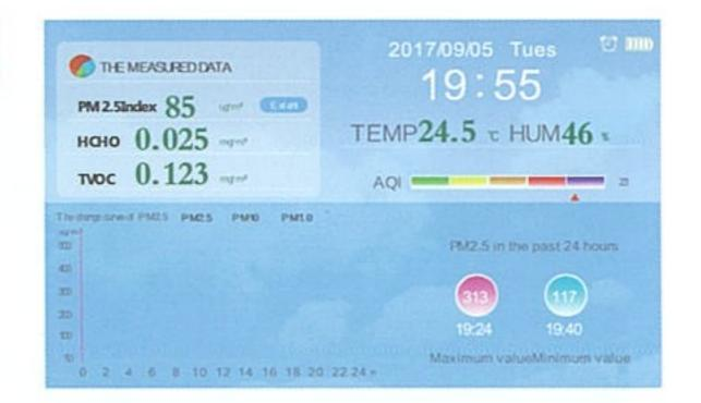
This interface display PM2.5, temperature, humidity. formaldehyde, TVOC, and AQI assessments. Press the SET button. the interface can be switched to display the value for PM2.5. PM1.0. PM10 test record value before 24 hours (record playback only save test data within the latest 24 hours after booting).
