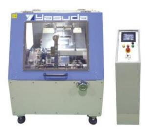
This tester is for evaluating the bondage of PVB film fragments inside safety glass composites used for automobiles.
