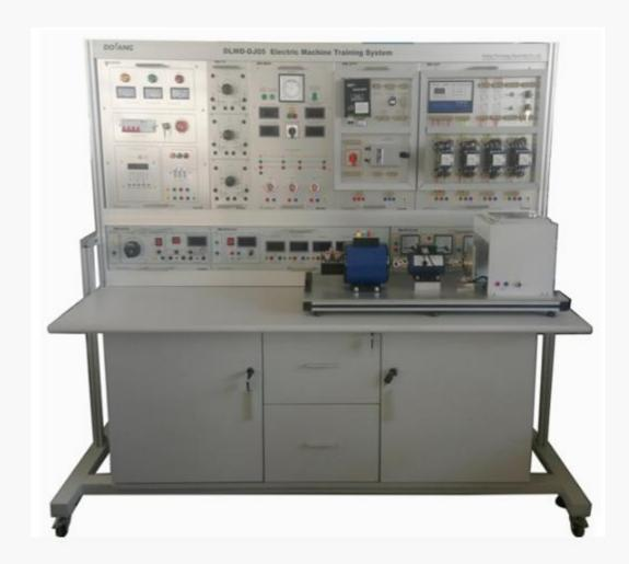
DLWD-DJ05 Electric Machine Training System consists of 10 different training motor, torque sensor, torque controller, magnetic powder brake, tension controller, various meters etc. Different motor control loop can be completed.
