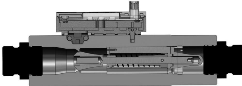
All FlowHUB's work on the same theory - the fluid flow is used to move a magnet which is mounted within a piston, the distance moved is proportional to the flow rate. This movement is measured by a sensitive magnetic device. The on-board electronics condition the signal and convert the linear movement to fluid flow. The FlowHUB also allows unmeasured flow in the reverse direction - when reverse flow is present the display will show '**-EE-**' ('**REV**' on ViscoCorrect version).
