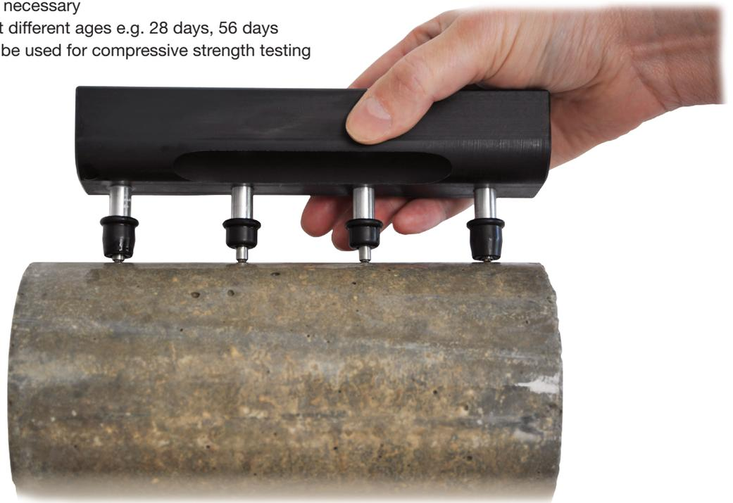
Resipod with 1.5" (38mm) probe spacing is fully compliant with the above mentioned standard
