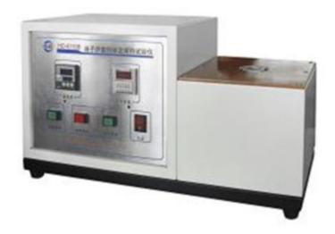
The HD-8110B type test machine is mainly used for the experiment of the terminal sheath resisting abnormal heat. The temperature setting range of the test machine is wide, the temperature is stable; the heating is stopped at the timing, and the alarm is given when the time is up.
