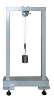
The insulation tightness test stand is developed with reference to relevant standards such as UL1581. It can test the insulation tightness of FXT, CXT and stranded XT wire cores; it can also test the insulation tightness of non-woven parallel cord power cores other than gold wire.
