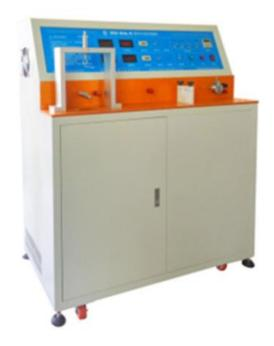
The broken beam and arc tester is a special equipment for testing the HPN type cord arcing experiment.
