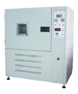
This instrument is mainly used for hot air aging test of rubber wire, PVC wire and other products, testing the aging extension and tensile strength of products and materials, and is suitable for quality control, laboratory and other places.
