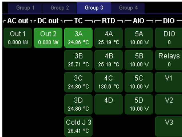
Now press the “Channel” button and touch the blue tab for the output channel that you want to use, “Out 2” in this example. You should see the channel setup screen for channel Out 2:
