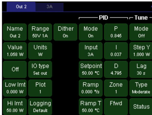
Select which temperature sensor you want to control: in the first “PID” column, touch the “Input” button. A window showing all available input channels appears. Touch the button for the temperature that you want to control, “3A” in this example. Sensor 3A is now the PID input for heater Out 2.
