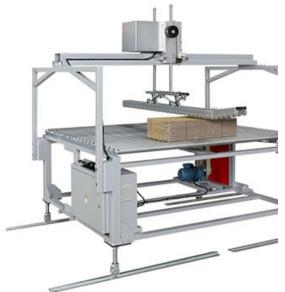
C-AC is an accumulating conveyor with press roller designed specially for corrugated industry. It functions as an accumulation/ buffer zone between strapping machine and upstream equipment, which allows one bundle to enter strapping machine at a time.
