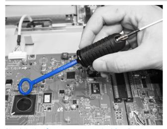
Pinpointing interference sources on a circuit board
